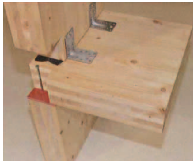
Fig. 17 – Bearing by Getzner (red, bottom) and Trelleborg (black, top) as possible improvement of the flank [7.7]
